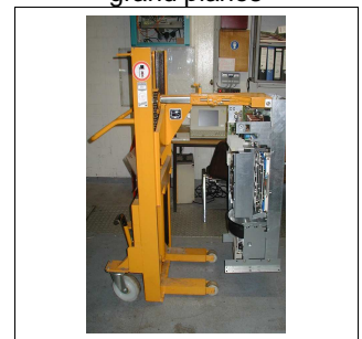
High lift stacker to assemble control cabinets
