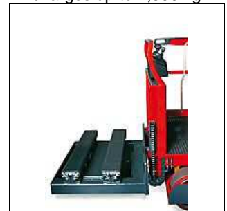
Very narrow aisle truck with telescoping fork
