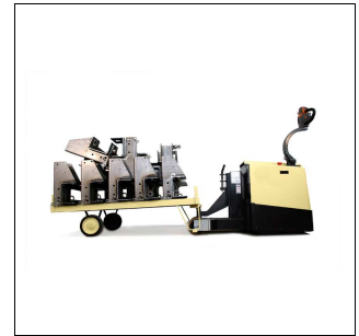
Heavy duty drawbar tow tractor (up to 20 to)
