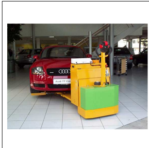
Electric low-lift truck to transport cars
