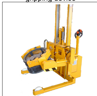
Electric high lift stacker for annealing baskets
