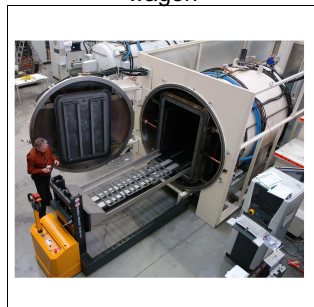
Electric lifting truck for loading ovens/Charging wagon in action
