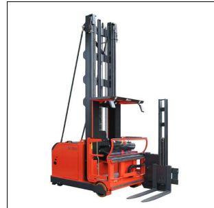
Very narrow aisle truck for charges up to 1,300 kg
