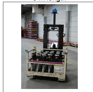
Driverless electric pallet stacker in action
