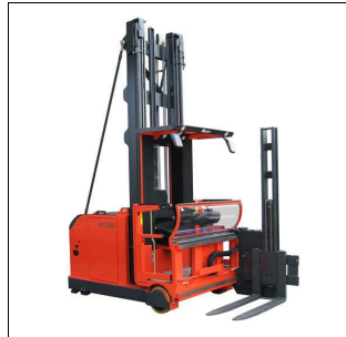
Very narrow aisle truck for charges up to 1,200 kg
