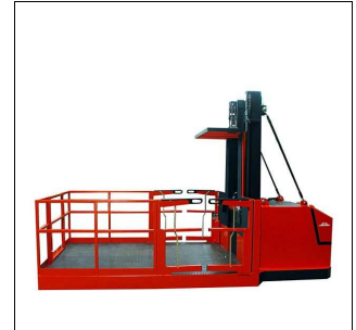
High level picker with platform
