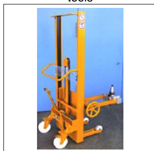
High lift stacker with tool changer
