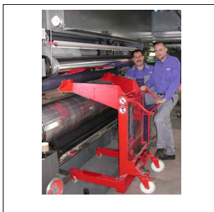
Equipment to lift out barrels
