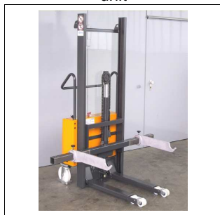
High lift stacker with pipe grab
