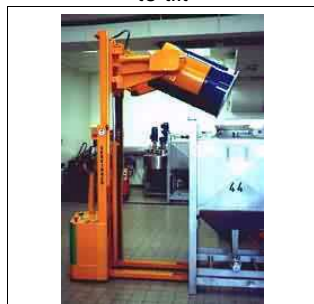
Electric high lift stacker with drum tipper
