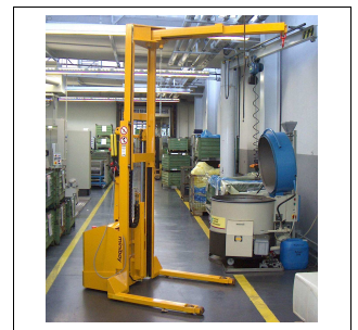
Electric high lift stacker with pivoting crane
