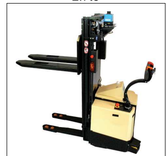
Driveless electric pallet in use as pedestrian truck
