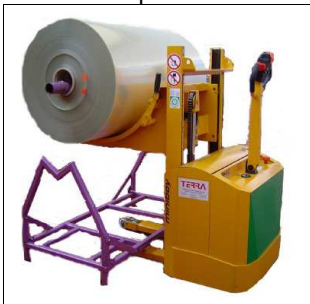
Electric high lift stacker with hollow to carry reels
